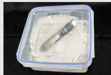
6. Close the box hermetically and wait for at least 4 hours. Check the value displayed by the hygrometer.
