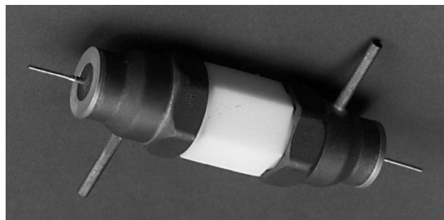
Fig. 3. Metal-insulator-metal resistor container of end copper fittings attached to middle PTFE sleeve.
