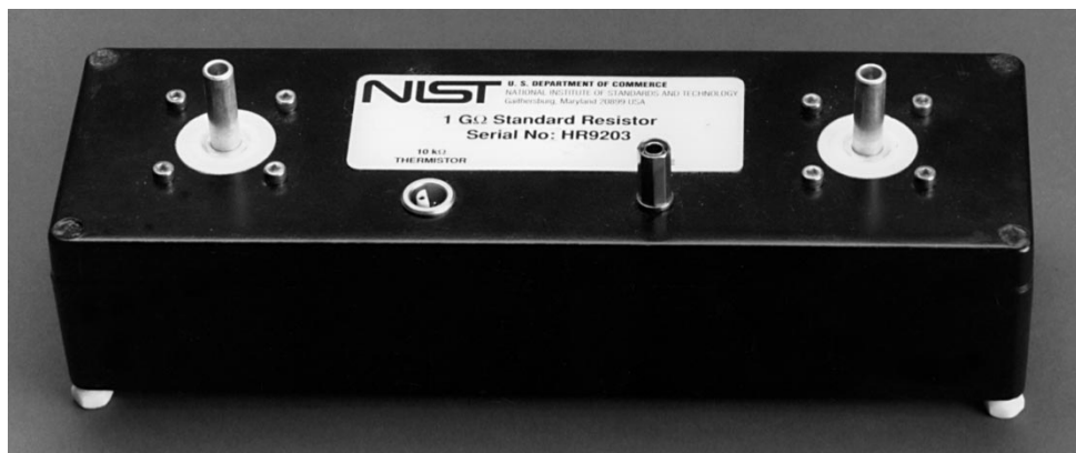
Fig. 2. Completed 1 GΩ standard resistor with coaxial terminals mounted on circular PTFE plates.
