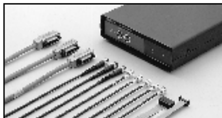
Model 5951 Remote Input Coupler: Includes the remote input coupler, five 1.2m low noise BNC cables (Model 4801), two 1m IEEE-488 cables (Model 7007-1), one 2m shielded IEEE-488 cable (Model 7007-2), and three 0.6m RG-58C BNC-to-BNC cables (Model 7051-2).
