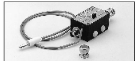
Model 6167 Guarded Input Adapter: Reduces effective cable capacity by driving the inner shield of the triax cable at Guard potential. For use with Models 220 and 224. 2-slot triax female to 2-slot triax male.
