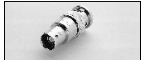
Model 237-BNC-TRX: Male BNC to 3-lug female triax adapter (guard disconnected). Terminates triax cable in BNC plug. High voltage rating for use with 237 and 7072-HV.
