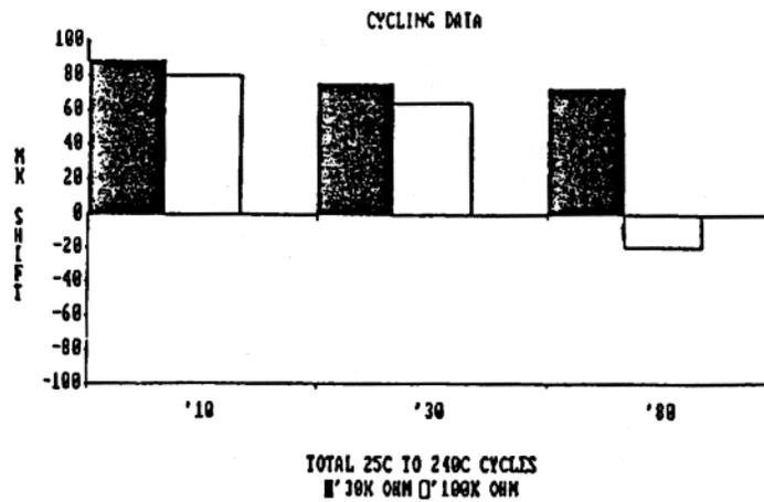
The results show no catastrophic failure. The small sample size may account for the variable behavior implied by the data.
