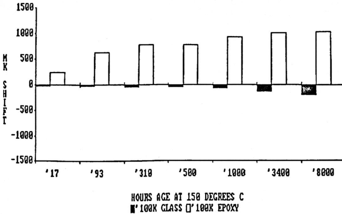
It is clear from these results that the glass encapsulation greatly improves drift characteristics for interchangeable thermistors at elevated temperatures.
