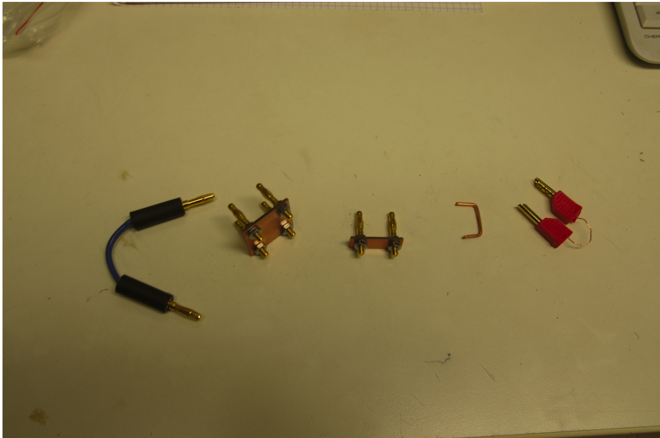
The tested short-circuit plugs. Sorted from left to right for decreasing stability. A certain thermal mass seems to be necessary to compensate for the temperature fluctuations of the air. All banana plugs have a gold surface, all cables are bare copper, no soldering. A science in itself, but one that should not be deepened at this point.
