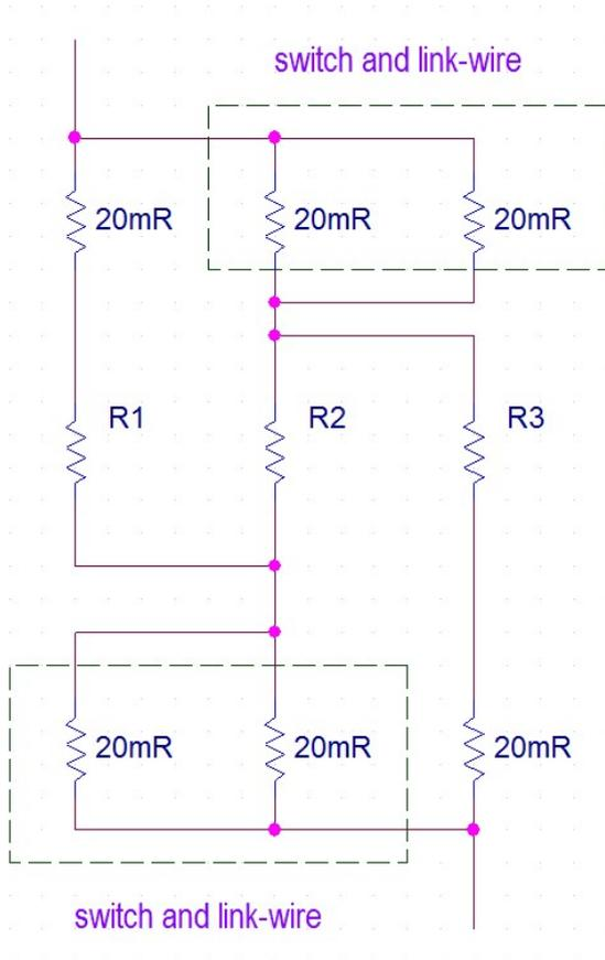
Here, the 10 mΩ switch and link-wire resistance has been split into two equal parallel paths, and the switch connection to R1 has been moved back along the interconnect wiring by 20 mΩ. Effectively each of the three paralleled resistors has gained 20 mΩ at each end. The calculation has been greatly simplified in the process.
