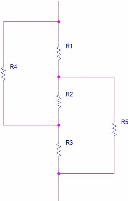
If we just consider the resistor chain in isolation, the parallel configuration has no internal leakage nodes. The series configuration has two leakage nodes, and we show them here with leakage resistances, R4 and R5, across the open series/parallel switch contacts.
