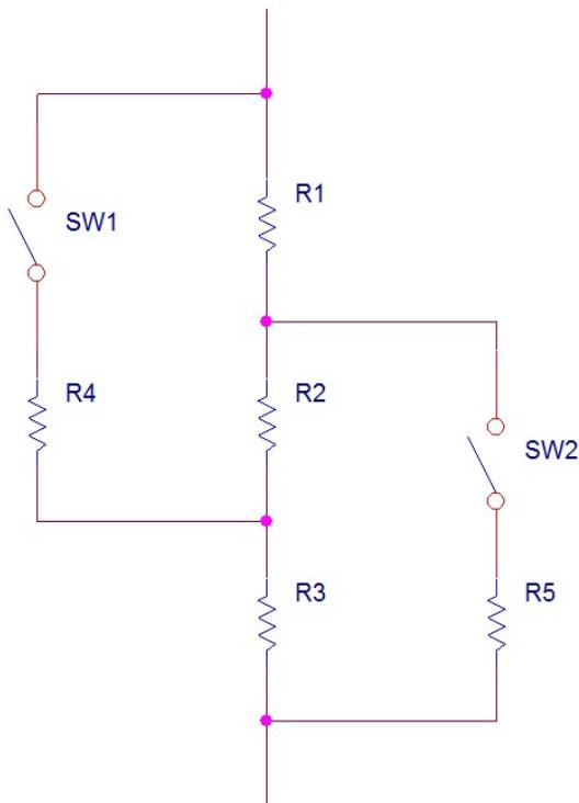
Sticking with the Fluke 752A scheme, it is not immediately obvious that the two switch contacts connect R1, R2, and R3 in parallel. Redrawing the circuit helps with this understanding.
