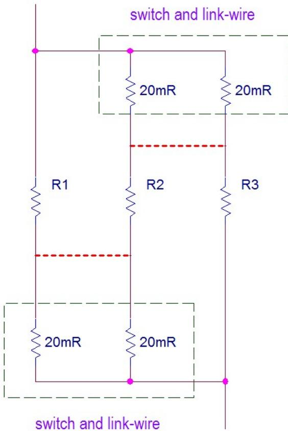
The 10 mΩ switch and link-wire resistances have been split into two equal parallel paths again, but this time we realise that there is (almost) no current flowing in the dotted red wires, so we can cut them (when looking at the parallel configuration)!
