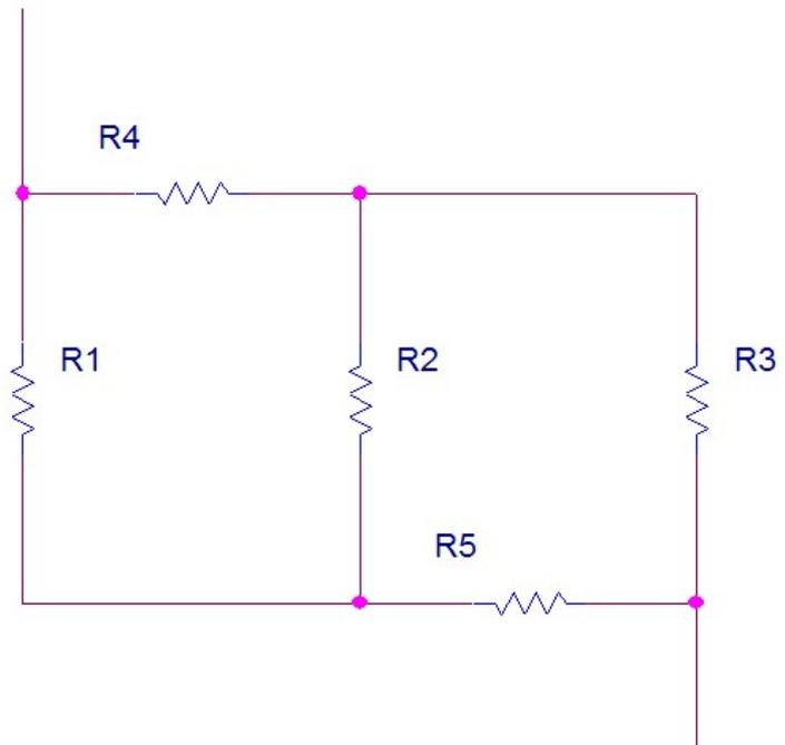
It is possible to accurately model this circuit with a circuit simulator, provided that the accuracy settings within the simulator are adjusted appropriately. R4 and R5 include not only the switch resistances, but also the link-wires necessary to join the nets together. To get a more intuitive model of what is happening we can re-draw the circuit again.
