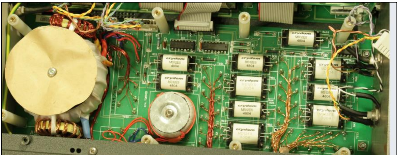
The three-stage ratio xformer (ratio 0.00 to 3.99) and tap selecting relays
