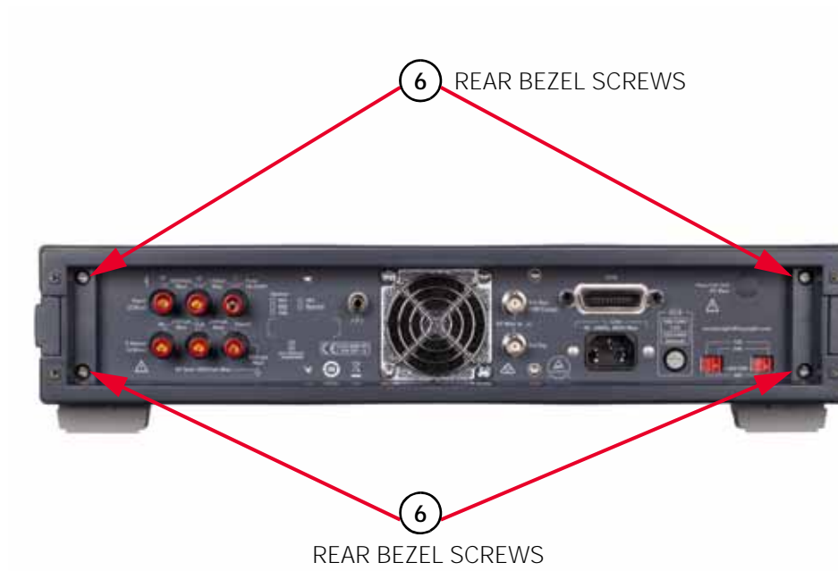
Figure 3-4 Remove/Install rear bezel
