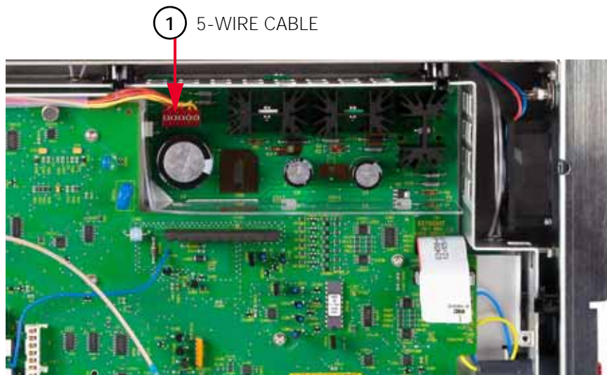
Figure 3-12 Remove/Install transformer cable on inguard power supply
