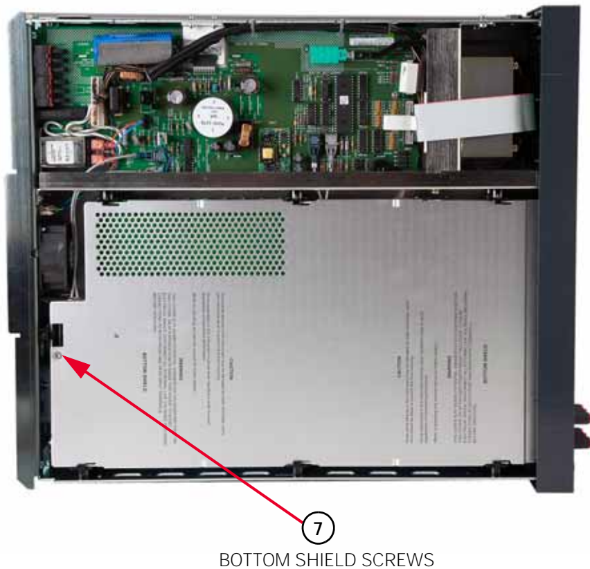
Figure 3-5 Remove/Install bottom shield screw
