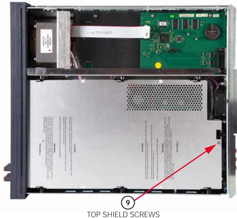
Figure 3-6 Remove/Install top shield screw
