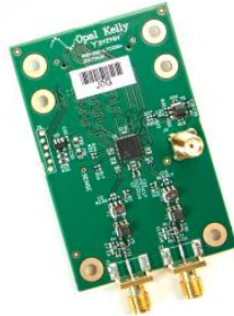
Analog-to-Digital Dual 40 MSPS, 12-bit
