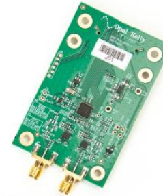
Digital-to-Analog Dual 125 MSPS, 12-bit
