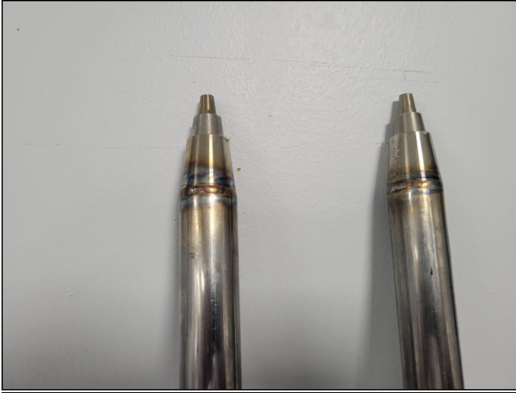
Figure 21 – TIG welding of nozzles
