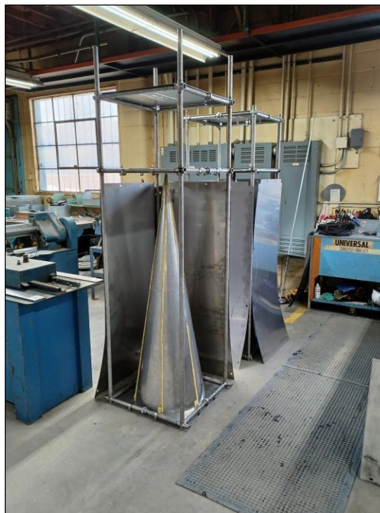
Figure 26 – Outer shielding for cone coils.
