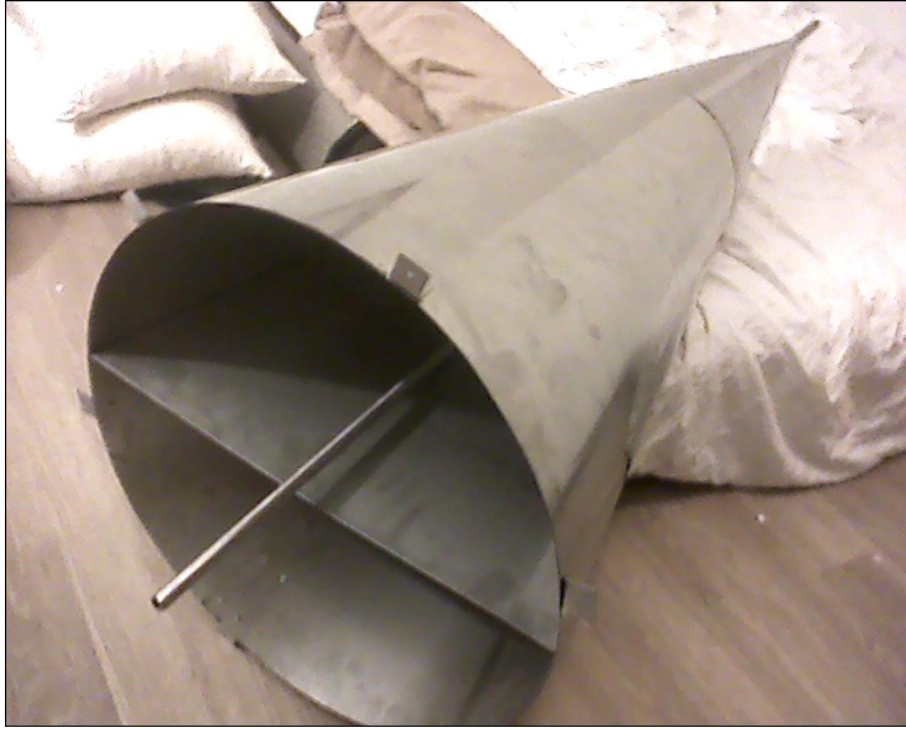
Figure 13 – bi-section of for inlet & outlet fans (air moves through a hole at the top of the bisection).
