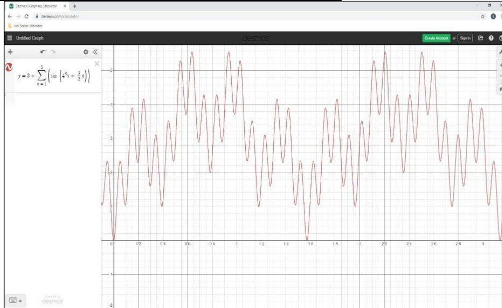
Figure 30 – Graph of 3 superpositioned frequencies.
