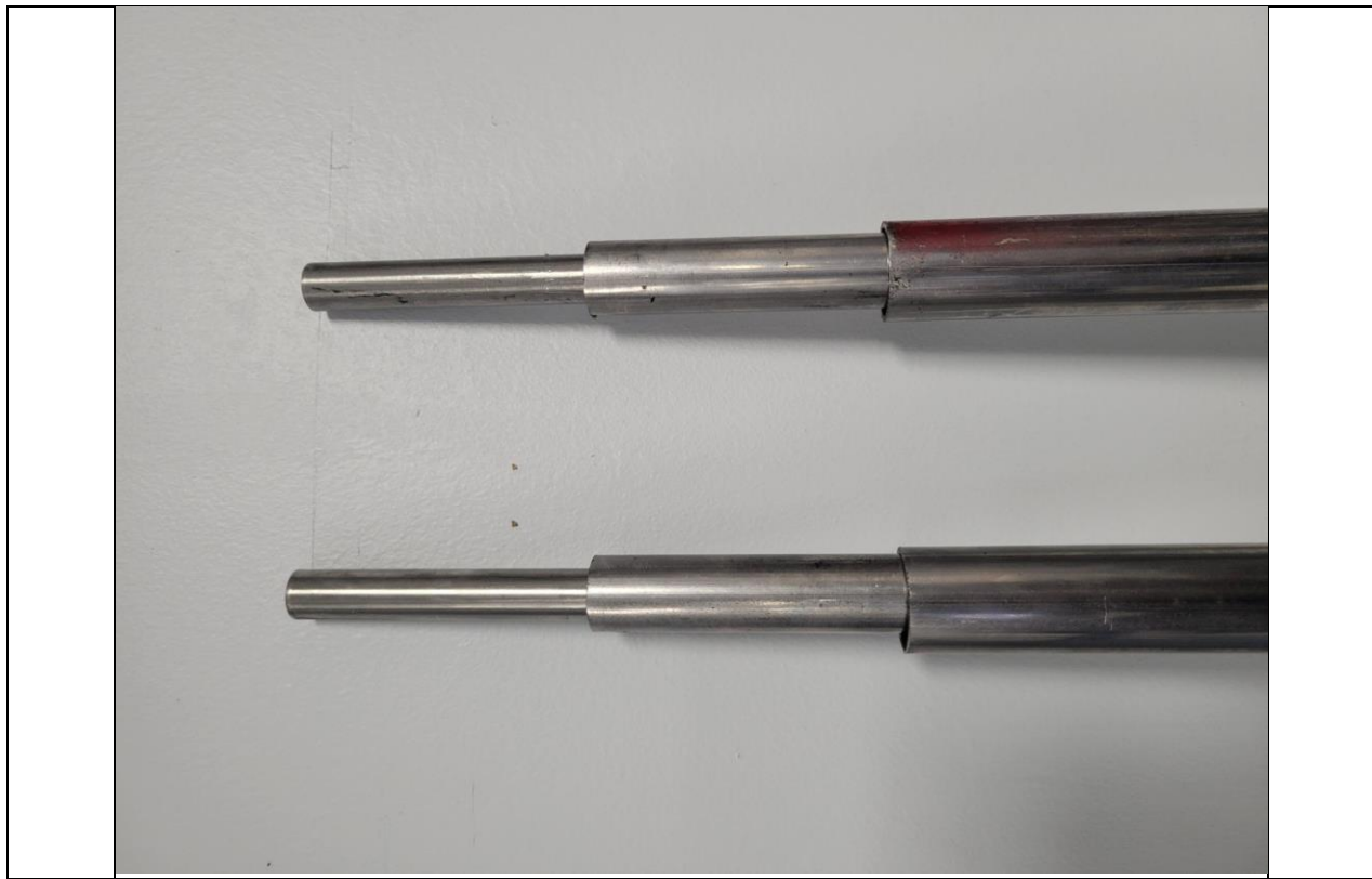
Figure 16 – Cut 304 Stainless Steel tubes – for nested-nozzles.
