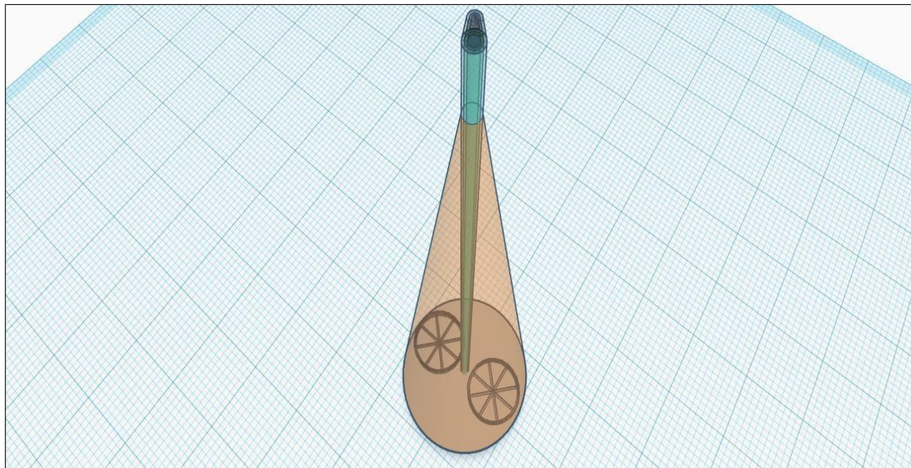
Figure 11 – CAD of inner helical nozzle/coil system, surrounded by cone coil.
