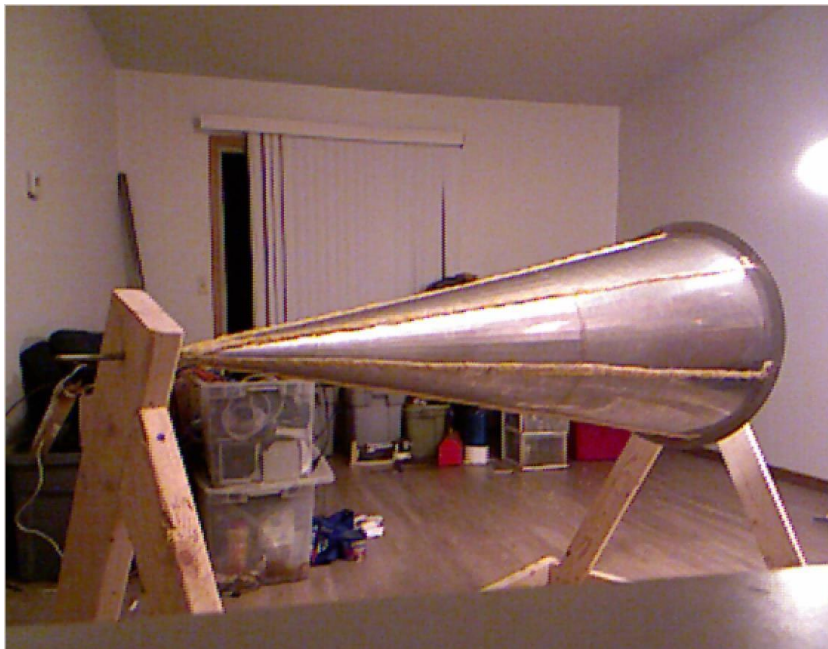
Figure 8 – wooden jig used for wrapping any coils (cones or helical)
