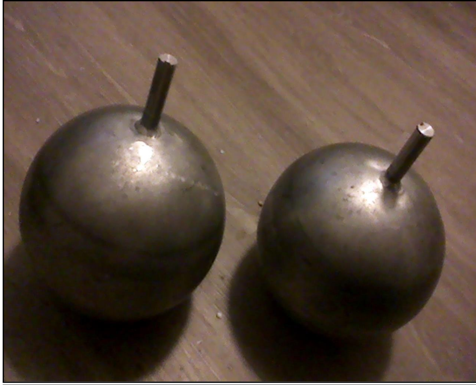
Figure 29 – TIG welded aluminum spheres and shafts (w/ keyslot).
