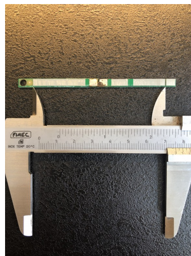
Fig. 3,4 -Antenna poorly soldered to the PCB – Length of desoldered Antenna
