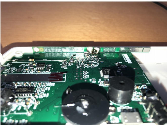
Fig. 3,4 -Antenna poorly soldered to the PCB – Length of desoldered Antenna
