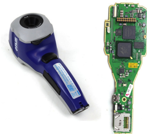
i7 Camera teardown (Courtesy of System Plus Consulting)
