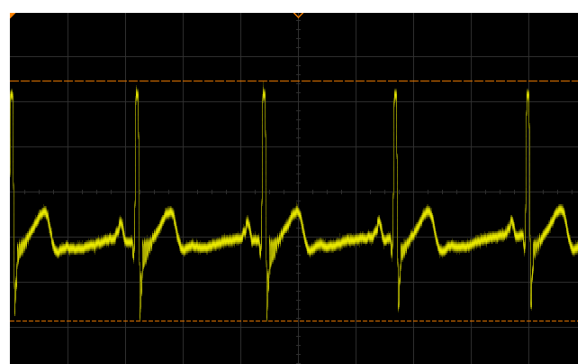
Figure 10: AFE module output when connected to a human subject in Lead II configuration using the Mason-Likar variant for electrode placement. (Normal Acquisition)
