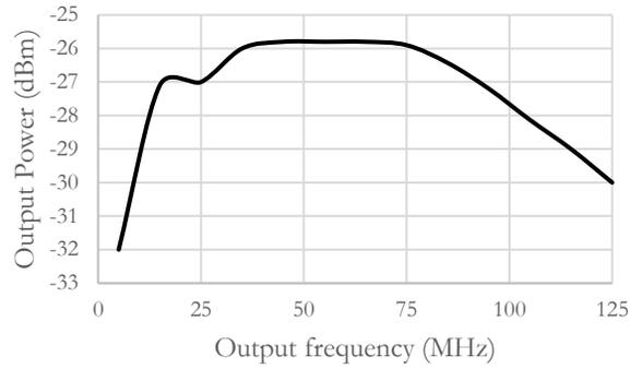
Figure 10: Downconverted Instantaneous Bandwidth of an input centered at 6 GHz with -60 dBm input power
