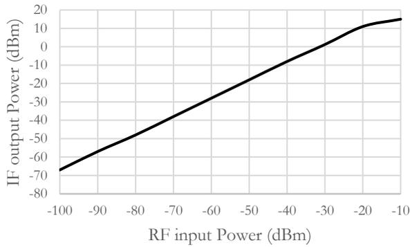
Figure 5: 75 MHz IF output power vs. RF input power at 8 GHz
