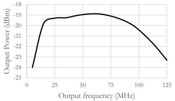
Figure 12: Downconverted Instantaneous Bandwidth of an input centered at 2 GHz with -60 dBm input power
