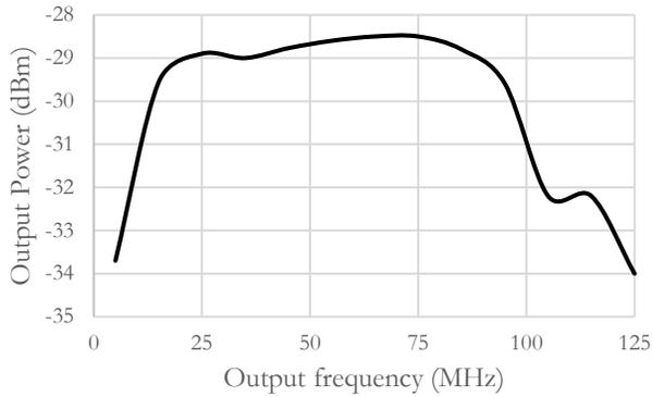
Figure 9: Downconverted Instantaneous Bandwidth of an input centered at 8 GHz with -60 dBm input power
