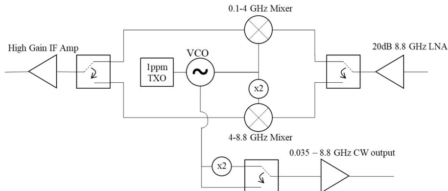
Figure 1: Simplified Block Diagram of the DGRF-8800Rx+'s Downconverting Receiver Path and CW Output
