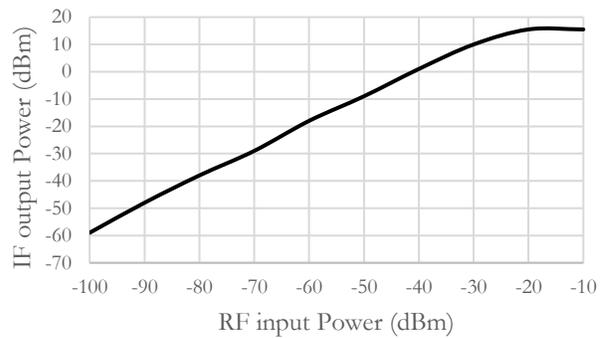
Figure 8: 75 MHz IF output power vs. RF input power at 2 GHz
