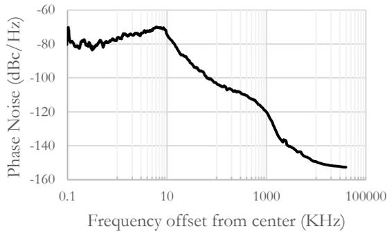
Figure 18: Phase noise of CW output at 4 GHz
