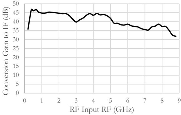
Figure 3: Receiver conversion gain vs. input RF frequency.
