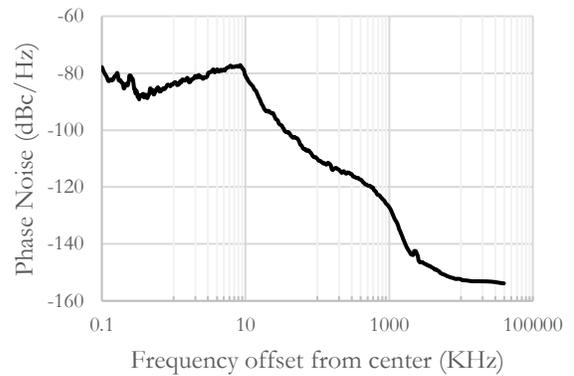
Figure 17: Phase noise of CW output at 2 GHz
