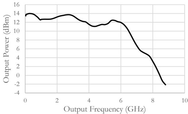
Figure 16: CW output power vs. frequency
