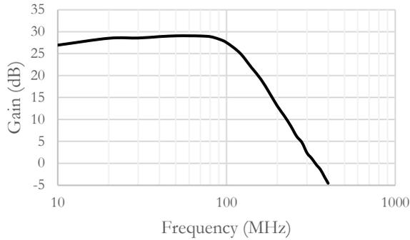
Figure 15: IF output IF Amplifier Gain vs. Frequency
