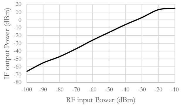
Figure 6: 75 MHz IF output power vs. RF input power at 6 GHz
