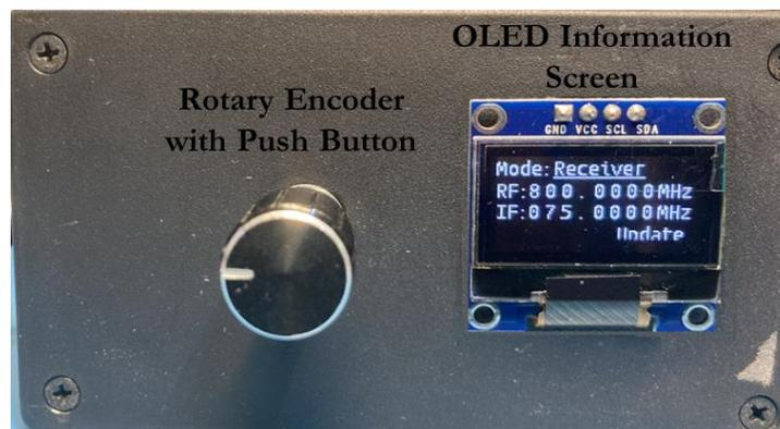
Figure 21: Photograph of the Rotary Encoder with Push Button Input and OLED display screen
