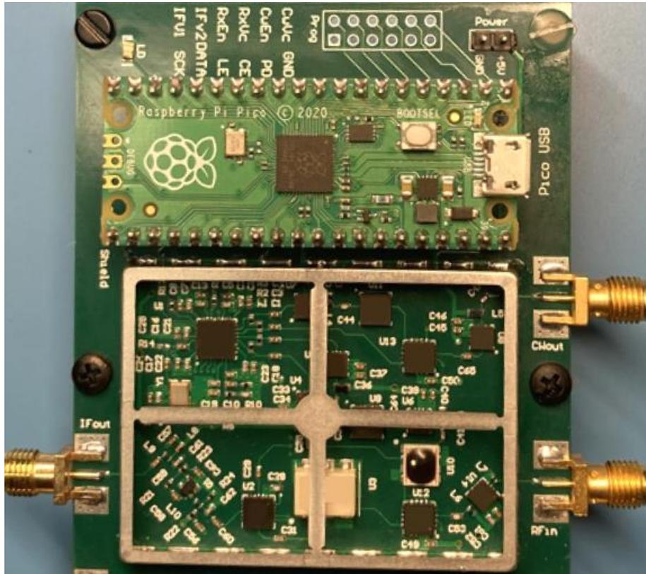
Figure 2: Photograph of Rev. A Circuit Board for DGRF-8800Rx
