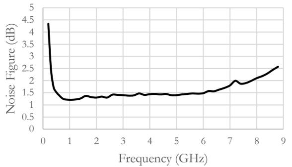
Figure 14: RF input LNA Noise Figure vs. Frequency
