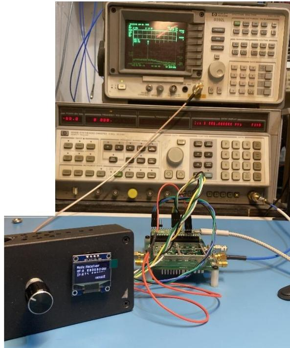
Figure 20: Photograph of DGRF-8800Rx+ under test along with its rotary encoder user interface and OLED screen
