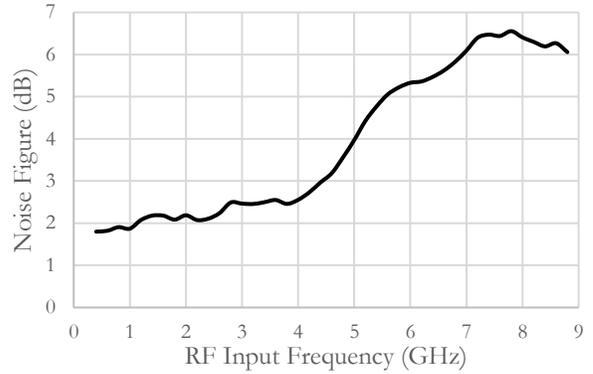
Figure 4: Receiver Noise Figure (NF) vs. input RF frequency.
