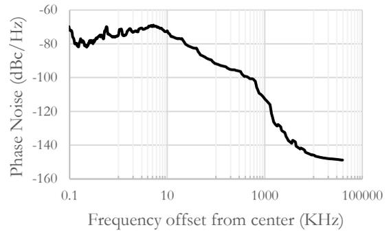
Figure 19: Phase noise of CW output at 6 GHz
