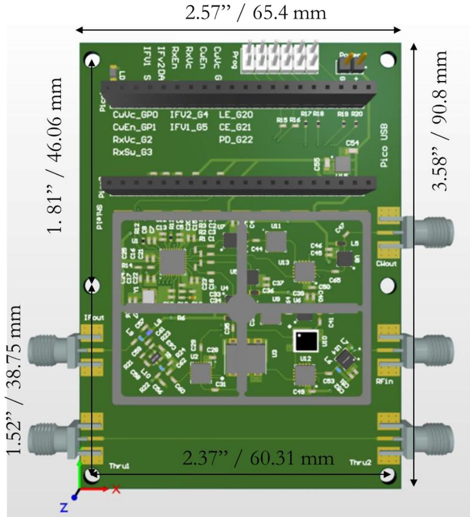
Figure 22: Dimensions for the initial prototype design for the DGRF-8800Rx+ PCB. When the product is transitioned to mass production the PCB will be altered slightly to eliminate the through line test ports and line. The mounting holes will be adjusted to fit the custom designed PCB housing.
