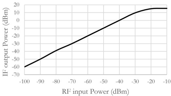
Figure 7: 75 MHz IF output power vs. RF input power at 4 GHz
