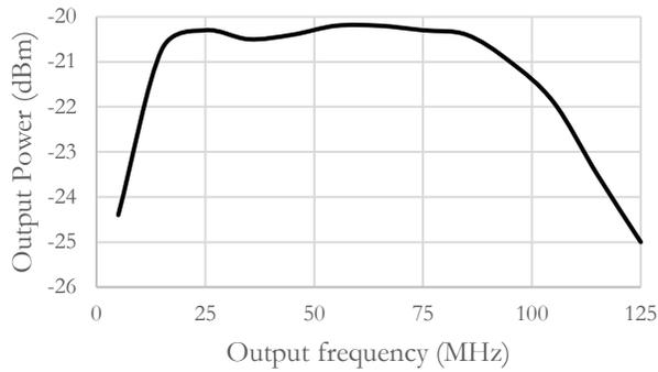
Figure 11: Downconverted Instantaneous Bandwidth of an input centered at 4 GHz with -60 dBm input power
