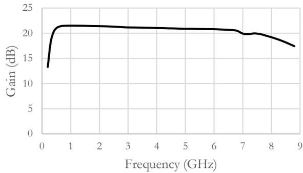
Figure 13: RF input LNA Gain vs. Frequency
