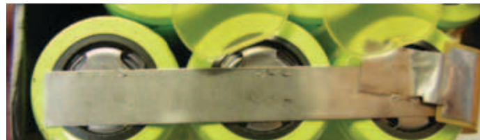
Insufficient welds that are not fully on the tabs
