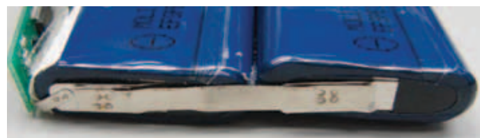
Half-moon shape of the welds indicate that the weld process used for this battery is not optimal
