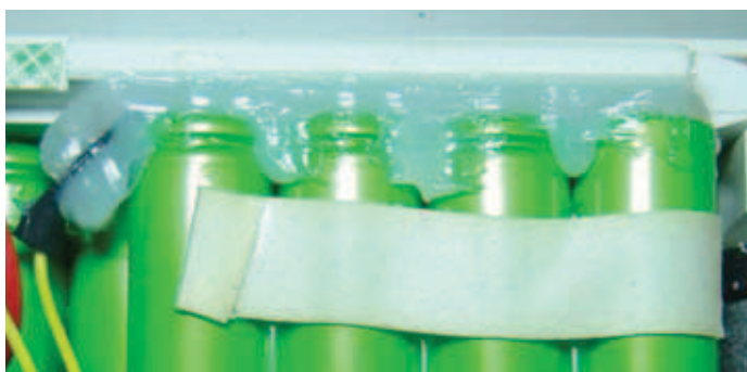
Excess silicone insulation can block safety vents
