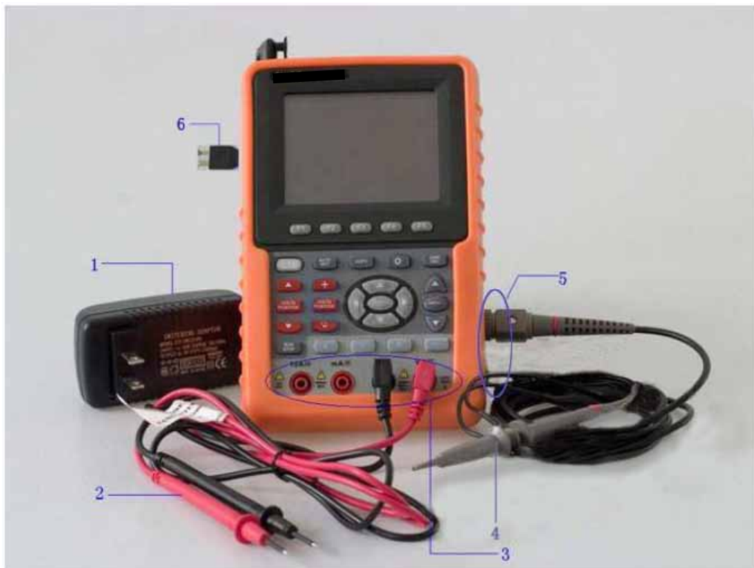
Figure 2: Input connections
