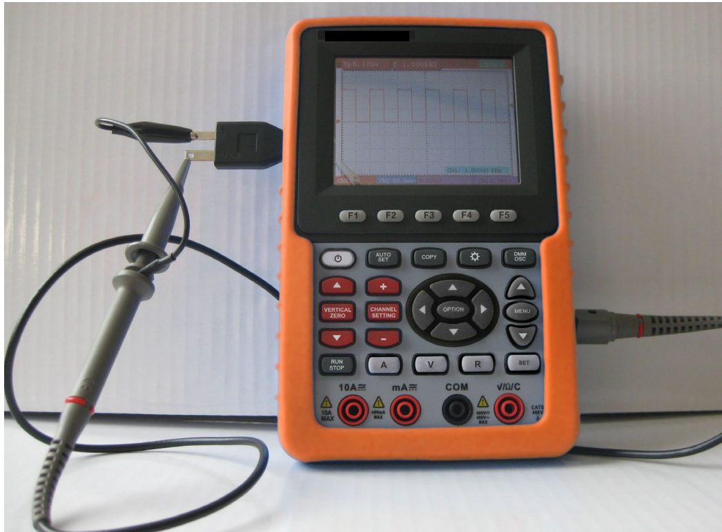
Fig.3. The connection of Square-wave test signal
