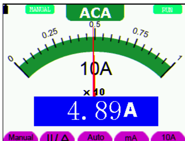
Figure 27: AC Current Measurement for 10A
