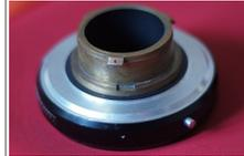
Mitchell 35R: 3 off, 1/4" wide prongs on a 42mm barrel. Flange focal distance = 56mm measured to sl prongs. Overall clearance between lens mount and gate = 42mm. The prong next to a locking slot is n Lenses: Super Baltars and Kowa. Picture shows a Hasslblad to 35R adapter. Likely early 35R camera
