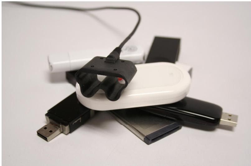
This device couples to the modem internal antenna signal and diverts it to a booster antenna thereby ensuring better signal reception and ultimately better communications.
