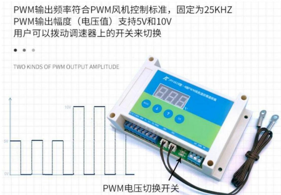
\*If you are not sure what voltage control signal the fan needs to adjust its speed, you can first turn the PWM voltage switch to 5V (the factory default is generally 5V). If the speed cannot be adjusted normally, turn the switch to 10V.
