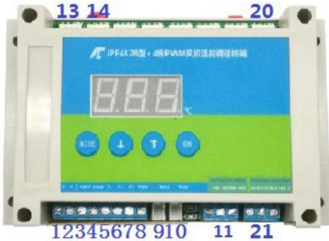
Terminal 1: Regulator power supply + pole interface; Terminal 2: Regulator power supply - pole interface,
