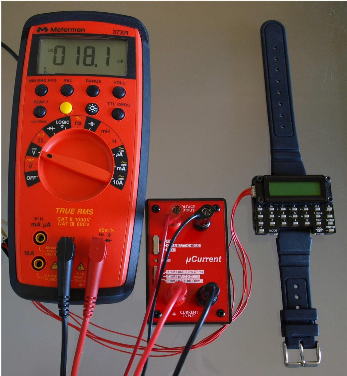
*Using the  $\mu$ Current to measure current drain of the author's  $\mu$ Watch.
