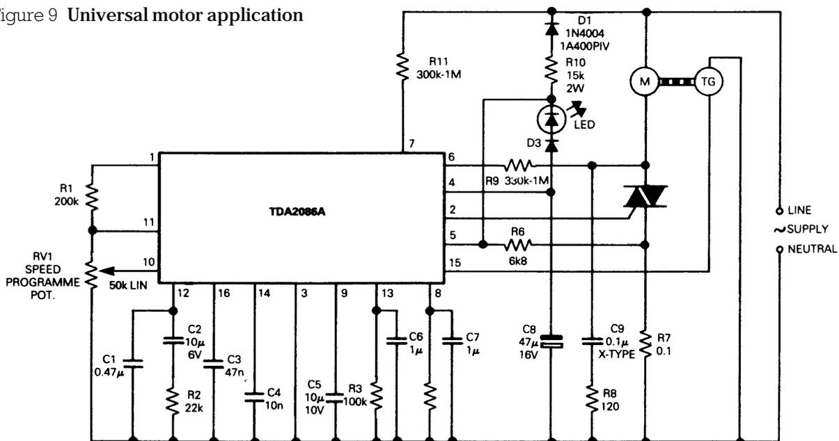
Note: A small capacitor may be required across the tacho coil to filter tacho noise at start-up.
