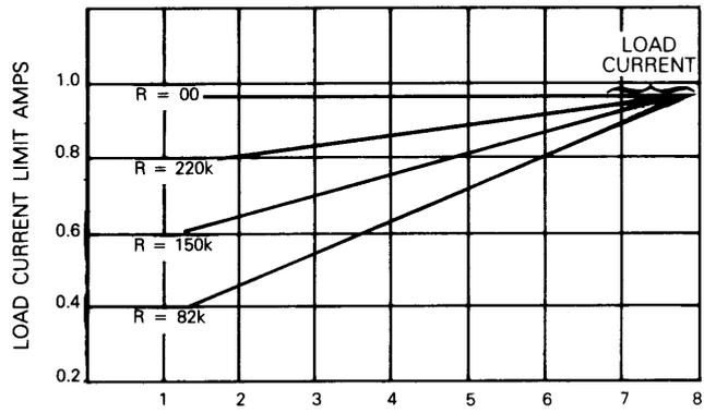
Figure 14 Current limit foldback, method 2
