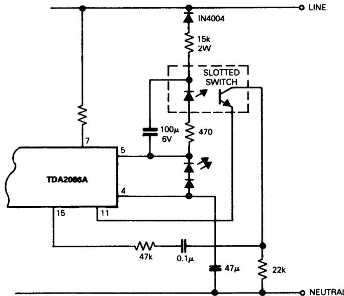
Figure 13 Current limit foldback, method 1
