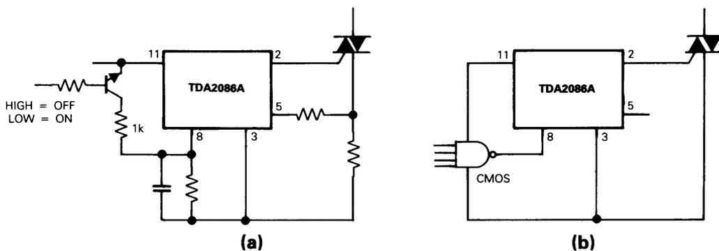
Figure 17 Temperature control application
