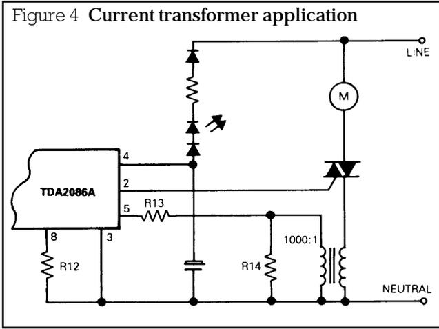
With a 1000:1 current transformer the average over-load current can be calculated from
