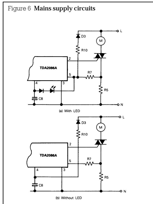
$$C8 = \frac{I_s}{V_{cr} \times f_m} \times 10^3 \mu\text{F} \quad \dots 13$$
